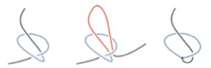
*Figure 1:* Schematic representation of various entangled structures discussed in this work (left to right): knots, slipknots, and lassos.
